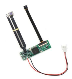
A camera module of a new generation with super low power consumption.
