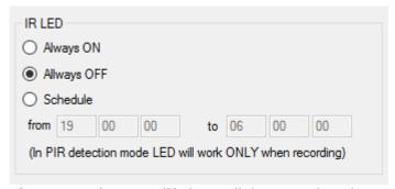
Always ON- The LED will light up all the time when the camera is recording.
