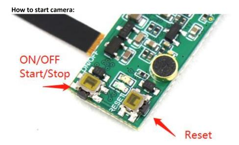
Press the button once and hold for 2 seconds, a yellow diode will light up.
